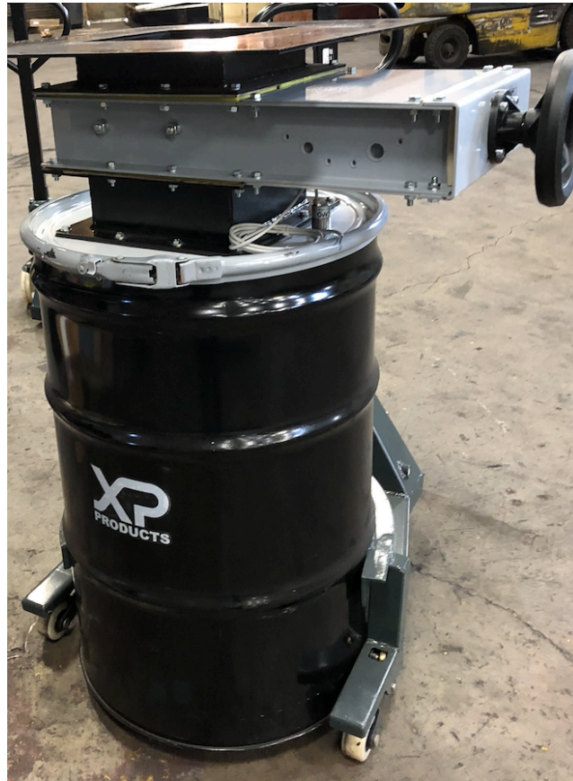
10''x10'' Square Gate with Manual Actuator
