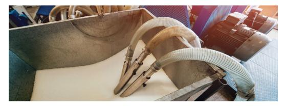
If, for example, a powder is poured out of a sack or conveyed through a pipe or hose any of the components can become charged. The same is true if the powder is sieved or poured through a hopper or of a liquid flowing through a pipe or hose.
