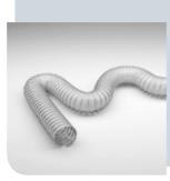
Suction & Transport Hose, laminated PTFE fabric, stainless steel helix, excellent chemical/weather • Oil mist extraction/suction resistance, good tear strength, hose wall nonstick material for optimum flow characteristics, highly flexible
