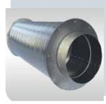
Sound attenuator, inner core perforated & corrugated aluminum, packed fiberglass insulation, outer core corrugated aluminum, mechanically fastened aluminum fittings on each end
