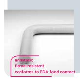
PU Suction & Transport Hose with stainless steel helix, ultra heavyweight, antistatic,  $R_0 < 10^9$ , flame-resistant, hose wall conforms to FDA, somewhat flexible, smooth inside for optimum flow
